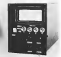
JET engine temperature analyzer unit consists of sensor-analyzer (left) and cathode ray tube indicator. Total weight of instrument unit is 6.6 lb.
